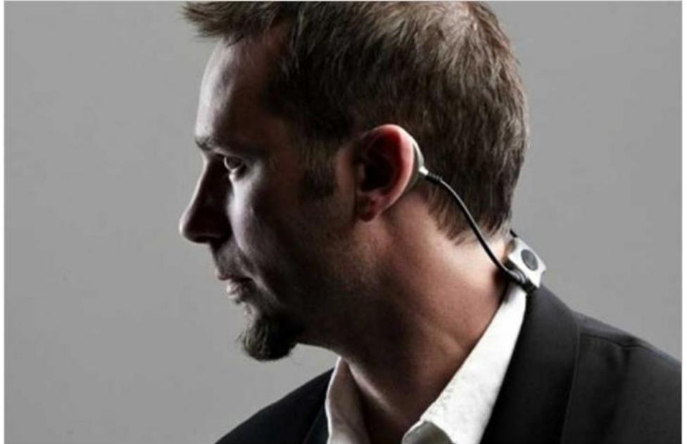
Basically, the headphones send tiny vibrations through the back of the ears, which is how the user is able to hear without blocking outside noise. Additionally, this method of transmitting sound makes the headphones silent to others, so users can listen as loud as they want without interfering in the lives of others.
