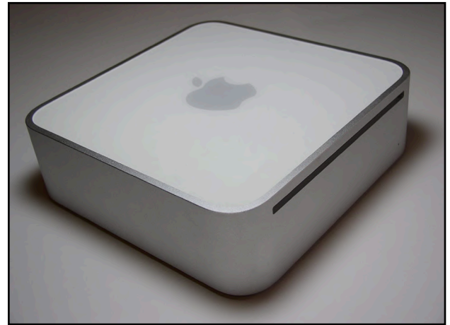
The original Mac mini desktop machine introduced in 2005 had an Intel processor inside. It was a hit with schools, ad agencies, video editors, and mainstream Mac users looking for the least expensive desktop Mac. Software called Rosetta allowed "old" software written for the earlier PowerPC processors to run.
